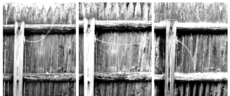
Fig. 4 Nail it on where you want it, but don't put it where the roof will drip on it, as it works with moisture from the air, not water on it.
